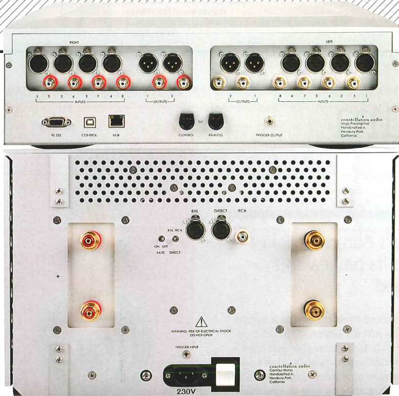
ABOVE: Constellation's Virgo preamp [top] offers four sets of balanced (XLR) and single-ended (RCA) ins with pairs of XLR/RCA outs. The network and USB ports are for control/updates, the other multipin sockets connect to the outboard PSU. The Centaur [bottom] has parallel 4mm speaker outlets, RCA and low/normal gain XLR ins
